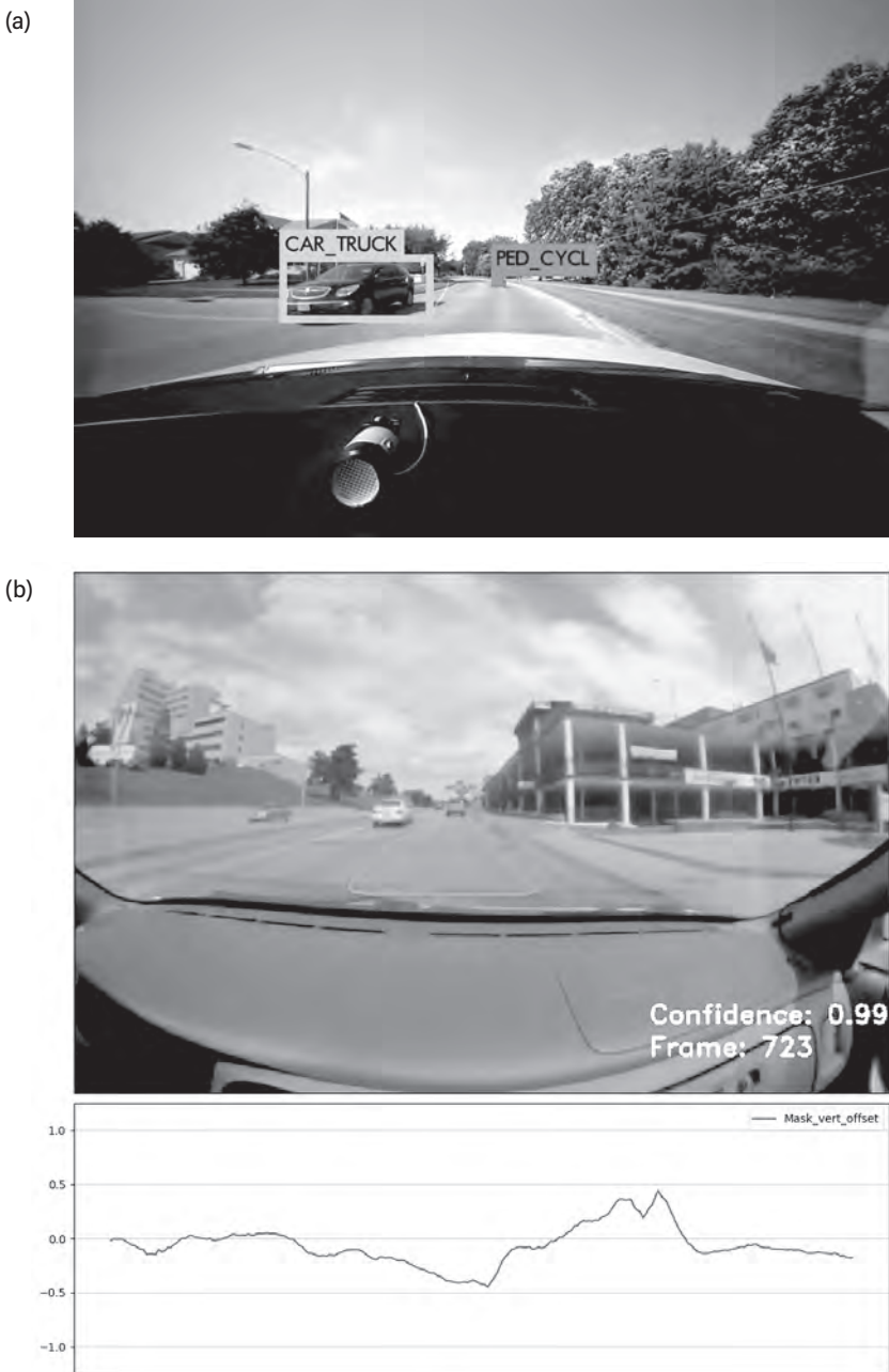
FIGURE 9.7. Computer vision algorithms can automatically process video data from thousands of miles of naturalistic driving data collection. Algorithms are trained on annotated data sets. (a) An example of detecting objects in the forward roadway, here a cyclist (PED_CYCL); the IV is following and a car (CAR_TRUCK) is in the opposing traffic lane. (b) An example of lane tracking. The outlined polygon in the forward roadway view shows the detected lane area, and the graph shows the vehicle’s detected lane position over time.
