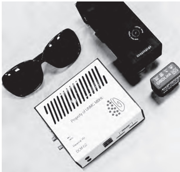
FIGURE 9.6. An example instrumentation system that can be installed easily and unobtrusively in a driver’s own vehicle. The white computer box (a) connects to vehicle power, coordinating the system and storing data. The black sensor package (b) contains sensors to record driver behavior. Additional sensor data is pulled from the vehicle’s on board diagnostic port (OBD) using a commercially available OBD device (c). Sunglasses are shown for size reference.
